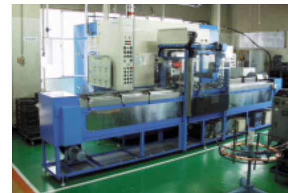
Non-chlorine organic solvent washing equipment (Headquarter Factory)
